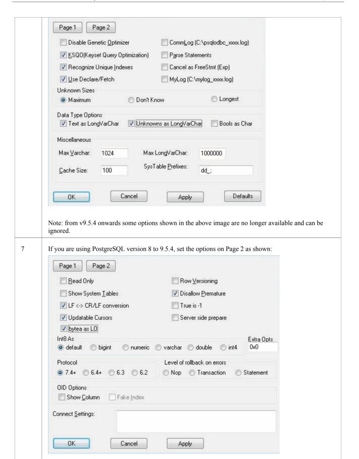
The 'Disallow Premature' checkbox should be checked
