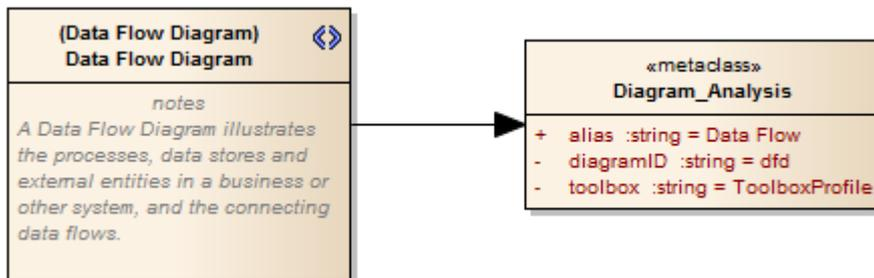
The Add Diagram Extension Profile Helper can assist you in defining your Diagram Profile, adding the necessary elements and giving them the appropriate attributes to define the functionality of the resulting custom diagram types.
