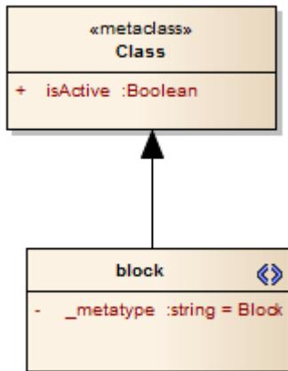
However, a SysML user is not interested in UML Classes, only in SysML Blocks. If you set the `_metatype` attribute to `Block`, any element created from that stereotype, while behaving like a stereotyped `Class` in most contexts will:
