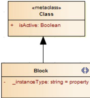
When a user drags a SysML Block element from the Project Browser onto a diagram, the system checks the `_instanceType` attribute value and searches the SysML Profile for an element template with a matching `_metatype` attribute value, and generates the instance from that - with the above definition you would get a Block element with the `<<property>>` stereotype.
