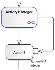
You can simulate this by setting a simple JavaScript statement to set the return value in the Activity's child element (such as this.return=12;) and, running the simulation, see the value transferred to the Action Pin in the Locals window.
