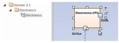
Select the 'Design > Element > Manage > Clone Element as New Version' ribbon option.
