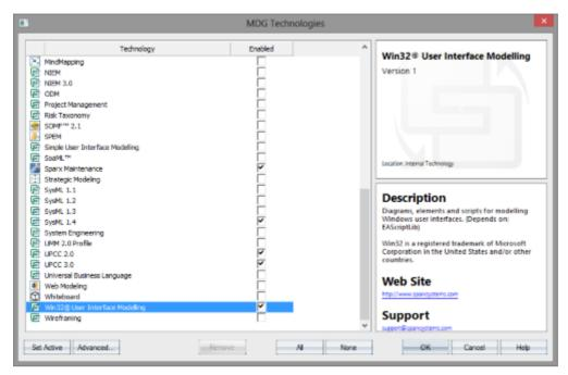
The Win32® UI Technology in Enterprise Architect is enabled or disabled using the 'MDG Technologies' dialog (select the 'Specialize > Technologies > Manage Technology' ribbon option).
