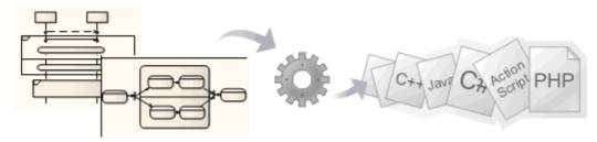
Enterprise Architect's multi-featured system engineering capability can be used to generate code for software, system and hardware description languages directly from behavioral models, such as StateMachine, Sequence (Interaction) and Activity diagrams. The supported languages include C(OO), C++, C#, Java, VB.Net, VHDL, Verilog and SystemC.
