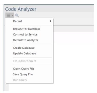
The menu provides various commands for activities associated with the use of the Code Analyzer, including such things as choosing a Code Miner database to use, updating the Code Miner database and Opening a Query File for editing.
