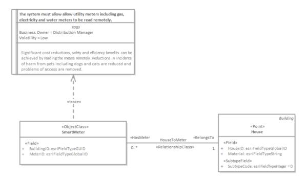
ArcGIS diagram showing a trace between a Smart Meter and a formal system requirement.
