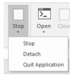
• Stop - stops the Debugger and stops the process that is being debugged (the default when you just click on the ribbon icon)
