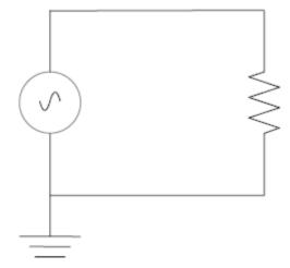
The circuit includes an AC power source, an earth and a resistor, connected to each other by electrical wire.
