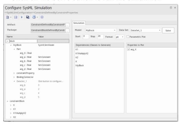
The result 120 (calculated as 2 \* 3 \* 4 \* 5) will be computed and plotted. This is the same as when we do an expansion with pen and paper: K = K1 \* K2 = (x\*y) \* (p\*q), then bind with the values (2 \* 3) \* (4 \* 5); we get 120.
