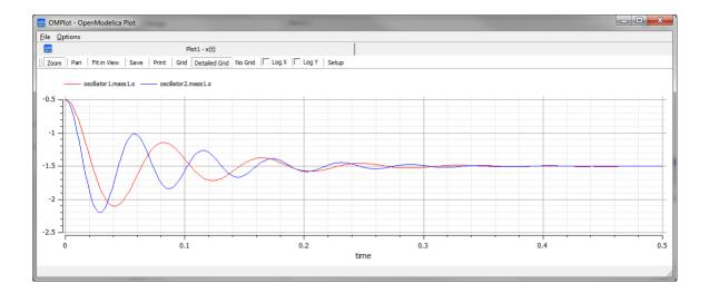
• Mass, light vs heavy: the object with smaller mass will oscillate faster and regulate more quickly
