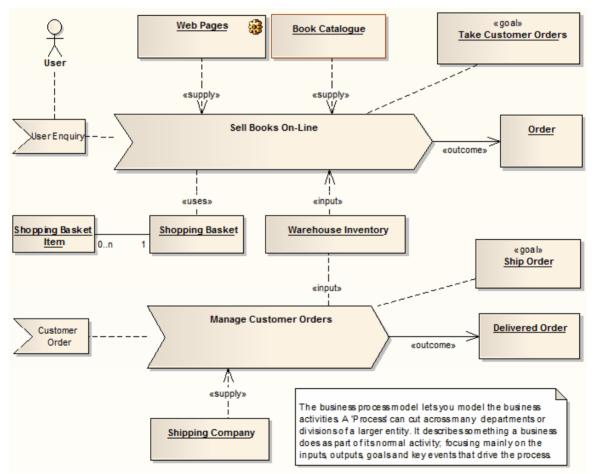
The second half of the process model is to respond to a customer order and ship the required items. The second process involves the warehouse inventory and shipping company, and completes when an order is delivered to the
