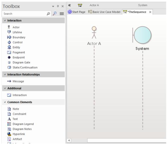
OK - we now have an Actor and a System and we want to represent the flow of Action and Response between the two entities. We can model this using messages between the two.
