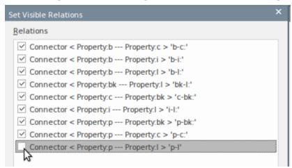
If a connector is not checked in this dialog it will not be displayed in the current diagram. It might, however, be visible in other diagrams where the connected elements are displayed. This can be set from the 'Layout > Diagram > Appearance > Visibility > Set Visible Relationships' ribbon option.
