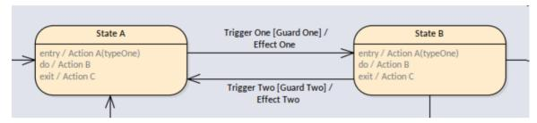
The transitions always originate from one State and target another, including the special case of a self-transition where the origin and the target are one and the same. The lines in the diagram have a label that can display a number of different options: *Trigger*, *Guard* and *Effect*. We will discuss these options in detail because they express important semantics about the transitions, including whether the transition will be executed at all. A transition can be in three conditions:
