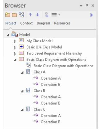
Double-click on the diagram link 'Basic Class Diagram with Operation' in the Browser window. This opens the diagram in the main workspace. Now, we will use the Features window to view the operations of Class A.
