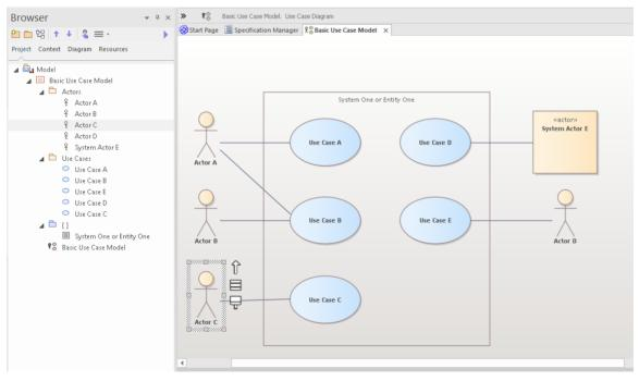
As you can see, there is an underlying model-level element in the Browser window that has a graphical representation in a diagram. Note that you can place a single model element in as many diagrams as you like, and that changing the name or notes or other element properties will be reflected immediately in all diagrams in which the element has been placed.
