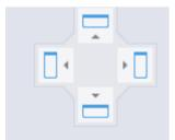
When you move the window over a compass point, an area of the display turns blue. This is the area that the window will occupy when you drop and dock it. You can then adjust the window borders to suit.
