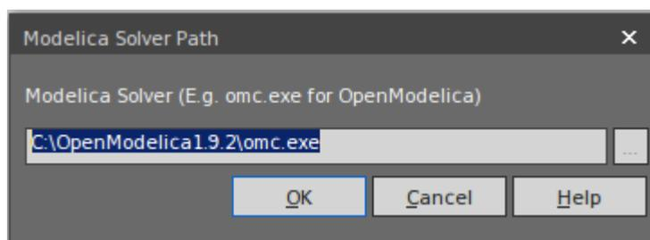
Type or browse for the path to the Modelica solver to use OpenModelica in Enterprise Architect.
