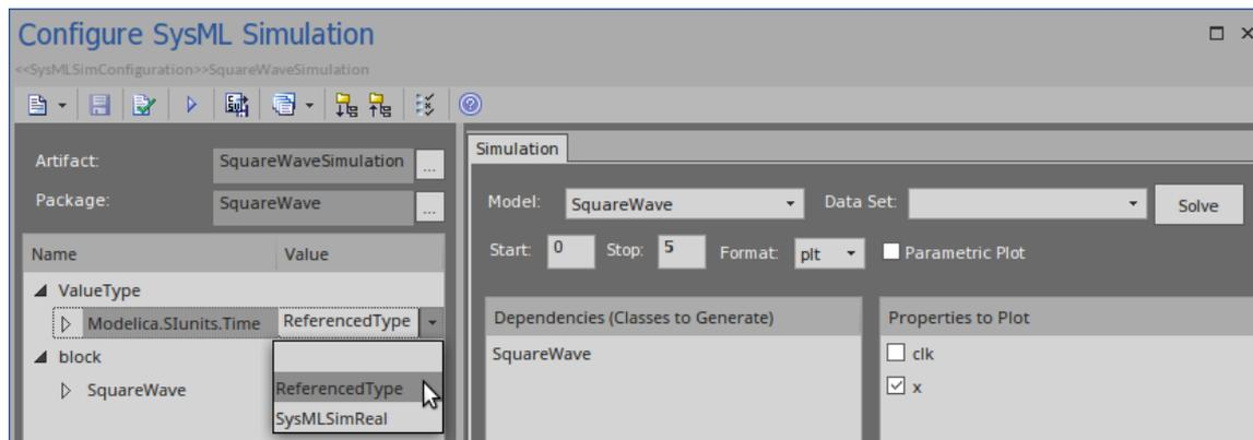
As the ValueType element is configured as 'ReferencedType', the element will not display in the 'Dependencies' list and will not be generated as a new Class definition to the Modelica file.
