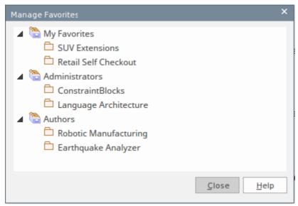
Right click on the Package to remove from the dialog, and click on the 'Remove' option. The Package is immediately removed from the list and is no longer flagged as a 'Favorite'.
