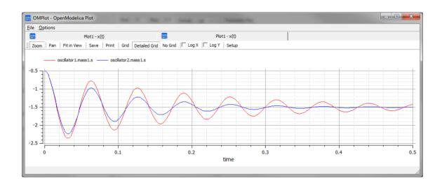
• Damper, no vs yes: the oscillator never stops without a damper
