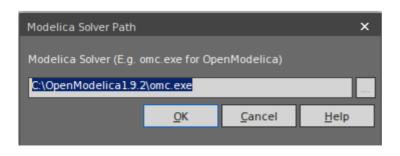
Type or browse for the path to the Modelica solver to use OpenModelica in Enterprise Architect
