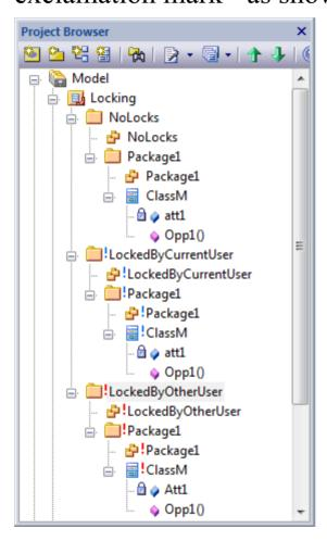
These indicators also display against the locked element on any diagram in which the element is represented.
