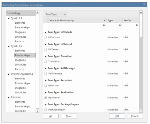
Click on the type of construct for each Technology in turn, and in the lists in the right-hand panel select the checkbox against each type of element, relationship, diagram, link rule or Pattern to allow in the Perspective. If it makes the process easier, use the All button or None button to select all checkboxes or clear all checkboxes before checking or clearing individual entries.
