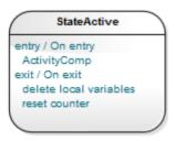
The operation Behavior is also applied during Interpreted Simulation and Executable StateMachine code generation and simulation, to provide 'entry/do/exit' behavior for States. In this case you create a short script in the 'Behavior' field, using JavaScript, to enact the operation behavior. For an example, access the EAExample Model and open 'Model
