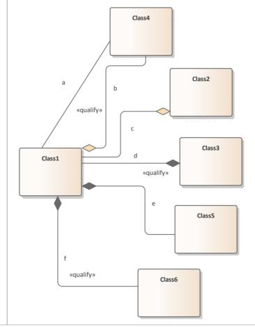
OR, if you right-click on connector **d** and select the 'Apply Line Style on Diagram | Connectors of the same SubType' option, you should see these changes to the connectors (only connectors **e** and **f** change because only those two are the same *type* and *subtype* as **d**, being strong Aggregations):
