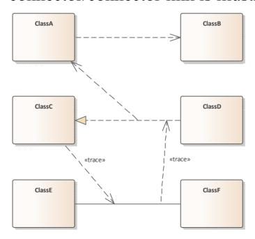
As you create the connector on another connector, the connector end displays with this circle symbol to indicate that it is on another connector, and to help you position the end accurately.
