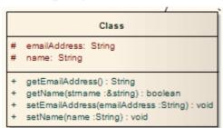
The example shows that, in the getName operation, the parameter 'strName' is a string reference, and is highlighted using the chosen character and position.
