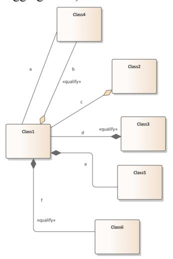
OR, if you right-click on Connector **d** and select the 'Apply Line Style on Diagram | Connectors of the same Stereotype' option, you should see these changes to the connectors (connector **f** changes
