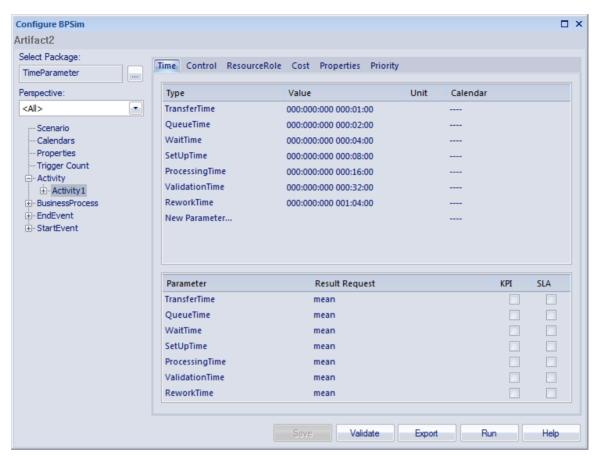
Note that in the upper panel there are seven system-supplied 'Time' parameters, which have been given initial values of in order - 1, 2, 4, 8, 16, 32 and 64 minutes (the 64 minutes is 1 hour and 4 minutes). Note also that in the lower panel, each of these has a Result Request for the mean runtime value of the parameter.
