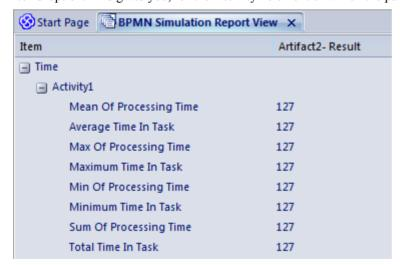
All of these derived results are 127 minutes, the sum of the initial values of the original seven 'Time' parameters. The individual parameters are not processed separately.
