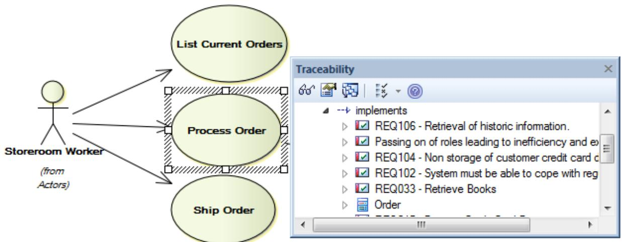
**Figure 16: The Traceability window showing this Use Case's requirement relationships**
