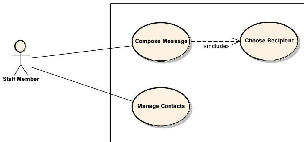
**Figure 34: Use case diagram showing actors and use cases.**
