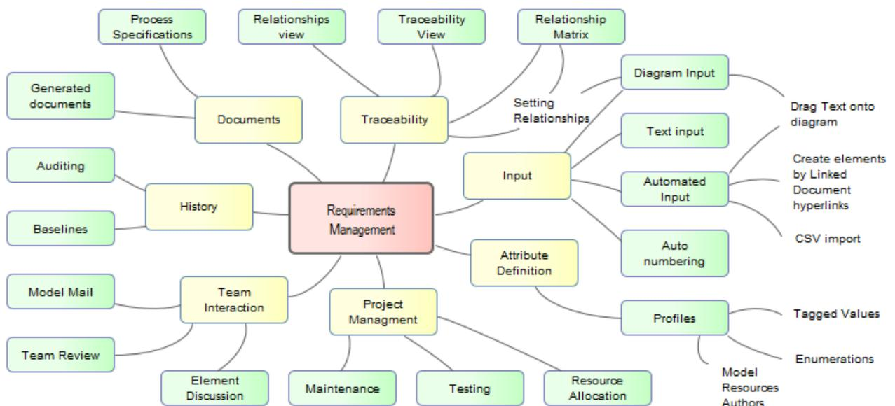
**Figure 1: Outline of the functionality that can be applied in Requirements Management**
