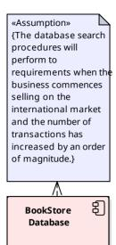
This diagram shows the use of an Assumption (constraint) that can be connected to an element to show some assumed condition. Constraints can be written informally in text or more formally in a language such as the Object Constraint Language (OCL).
