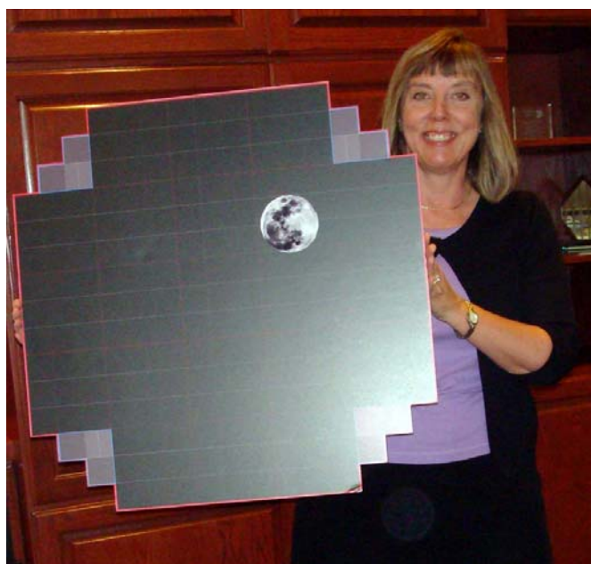
Figure 1. Suzanne Jacoby with the LSST focal plane array scale model. The array's diameter is 64 cm. This mosaic will provide over 3 Gigapixels per image. The image of the moon (30 arcminutes) is placed there for scale of the Field of View. (Image credit: LSST Corporation)
